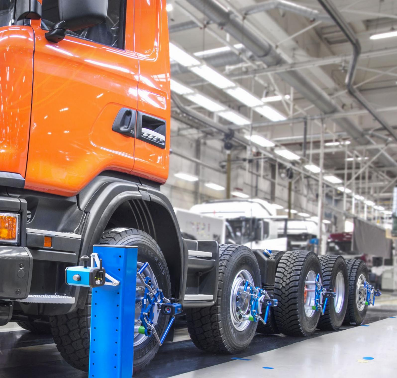
**THE ACTUAL MEASUREMENT** process starts as the operator aims the camera forward, clicks the OK-button, turns the camera to point backwards and clicks again.
